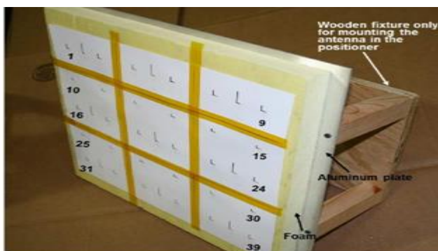
Fig. 10. Fabricated dual-band array
