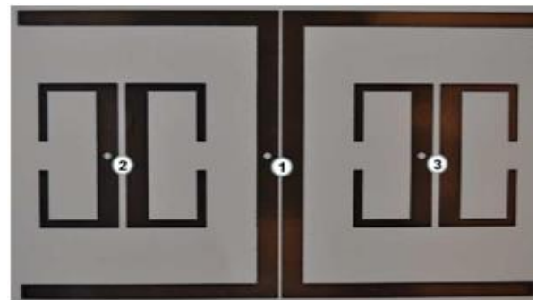
Fig. 4. Fabricated nested antenna element
